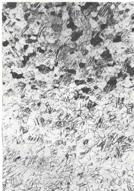
59 Shocked zone in iron. \times 80 .
