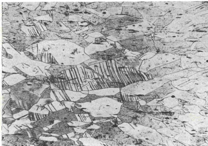
57 Mechanical twins in explosively welded copper. \times 200 .
